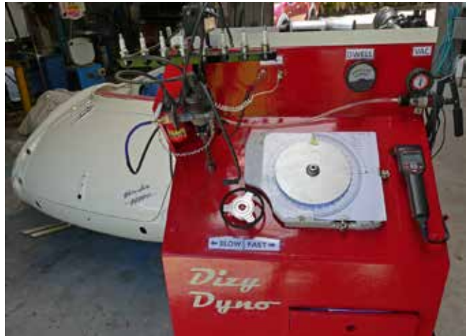
Distributor test bench for analysing distributor performance.
